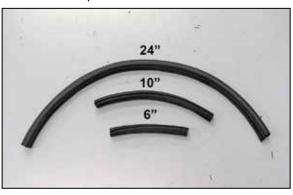
9. Cut the provided edge trim into three sections as shown. One section will be 6" long, one will be 10" long and the last one will be 24" long.
