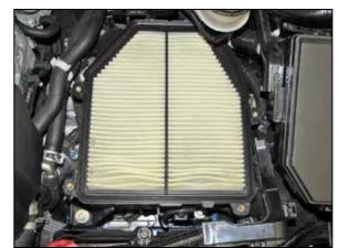
6. Remove the factory air filter.
