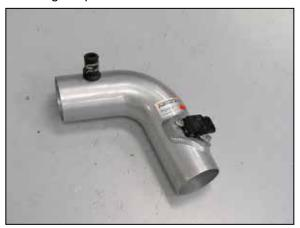
19. Install the provided grommet into the K&N<sup>®</sup> intake tube along with the factory crank case vent spring clamp.
