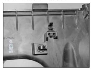
13. Remove one of the transmission vent hose clips from the lower air filter housing.
